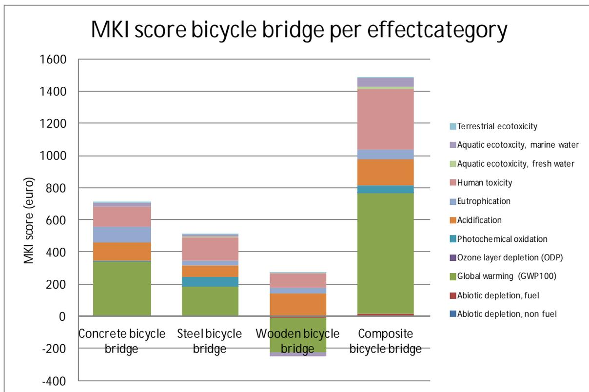
The environmental impact expressed in MKI score of the bicycle bridges varies greatly. The wooden bike bridge has a very low MKI score. The MKI scores of concrete bicycle bridge is slightly higher than that of the steel cycle bridge and about half of the MKI score of the composite bridge.
