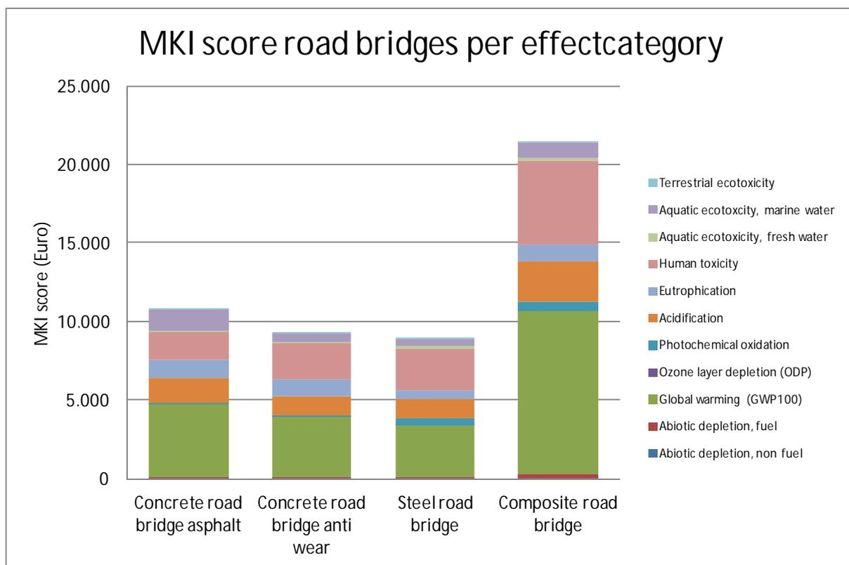
The results of the road bridges are largely similar to the bicycle bridges: The MKI score of the steel and concrete bridges are similar and the MKI score of the composite bridge is about double this score.
